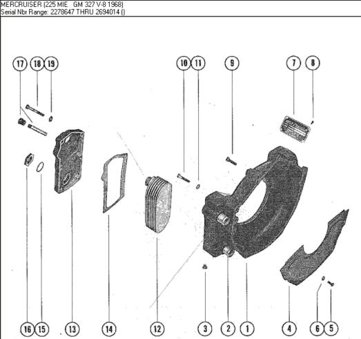
FLYWHEEL HOUSING AND OIL COOLER (INBOARD)
